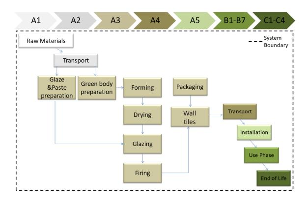
Flow chart of manufacturing walltiles and LCA system boundary.
